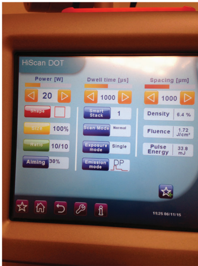
FIG. 6. Specs for lichen sclerosus CO 2 laser treatment are: power, 20 Watts; time on tissue/emission, 1000 microseconds; and interval, 1000 micrometers.
